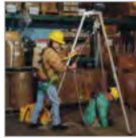
A secondary fall arrest system is recommended
