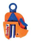
The IPNM10P vertical lifting clamp is used for the lifting, turning, moving or vertical transfer of sheet, plates, or fabrications from horizontal to vertical and down to horizontal (180°) as needed without marring the surface of the material. Materials such as aluminum, stainless steel, painted materials, aircraft skins, composite material, glass, plastic, etc., can be lifted without marring. The protective cover reduces the risk of damage to surrounding plates.
