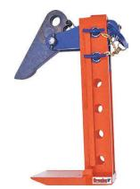
The IPPE is suitable for the lifting and transfer of bundles of non-sagging steel plates in horizontal position. The jaw opening can be easily adjusted. Raising the handle opens the clamp. This facilitates the easy and quick placing or removing of the clamp.
